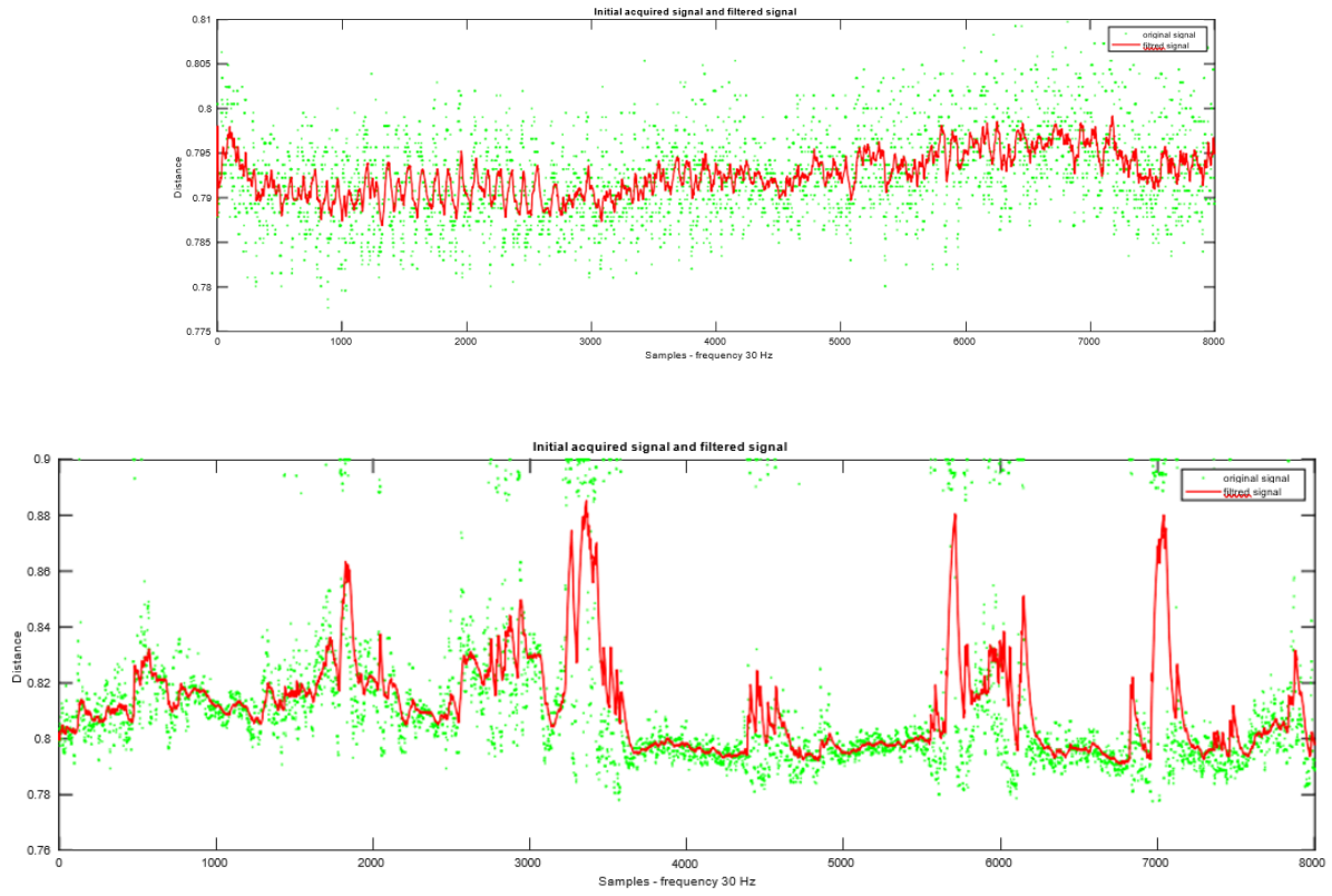
Figure 4. Initial acquired signal and filtered signal - frequency 30 Hz (a) Measurement performed when a person is breathing normally (b) Measurement performed when a person is breathing abnormally
