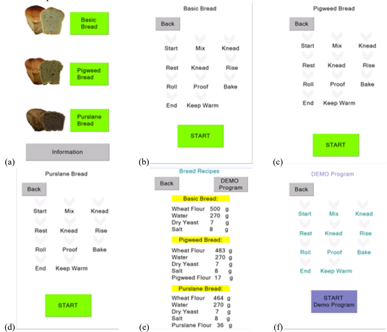
Figure 8. Screens of HMI. (a) Main screen; (b) Basic bread screen; (c) Pigweed bread screen; (d) Purslane bread screen; (e) Information screen; (f) Demo program
