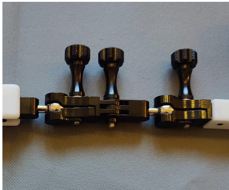
Figure 13. The articulated aluminum arm used for alignment first and then for locking with the screws provided
