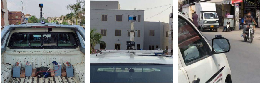
Figure 2. A glimpse of the camera and power backup setup on the data collection vehicle
